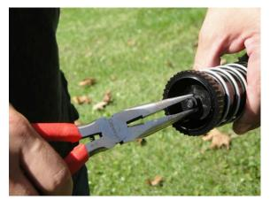
The filter on the bottom of the internal assembly can be easily removed using needle nose pliers.
