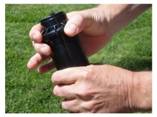
Unscrew the body cap counter clockwise, sometimes after use pliers may be necessary to free the body cap from the rotor's body.
