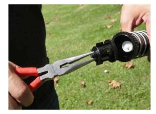
Generally, if cleaning the filter does not solve non-rotation then the sprinkler must be replaced.
