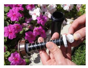
Another reason may be water leaking through the valve, because it is not completely closing. Typically, water will leak through a valve because debris is in the valve. To fix this, you'll need to disassemble the valve, rinse all the parts with clean water, and reassemble the valve.
